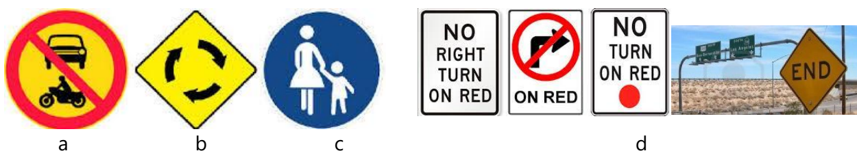
Fig. 6. Road signs: a – Motor vehicle traffic ban, Finland; b – Roundabout, Ireland; c – Pedestrian zone, Germany. Icons are depicted using dot, silhouette and linear graphics in certain color combinations [13]; d – Signs with using fonts, USA [10]
